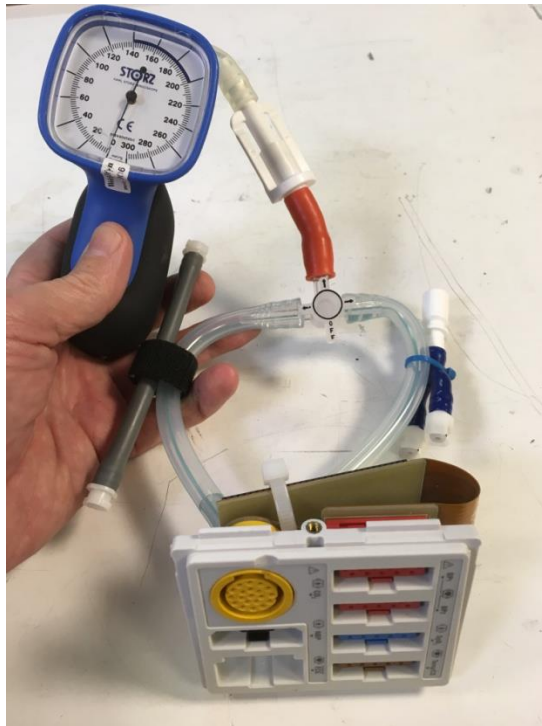
I can attach a BP hose directly to this and do a leak check, or let the MD do a manual BP.
